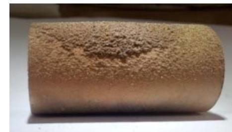
$$CE = \frac{m_{Dep}}{m_{Ash} \frac{A_{mullite}}{A_{reactor}}} 100 \quad [\% \text{ kg}_{Dep}/\text{kg}_{Ash}]$$
